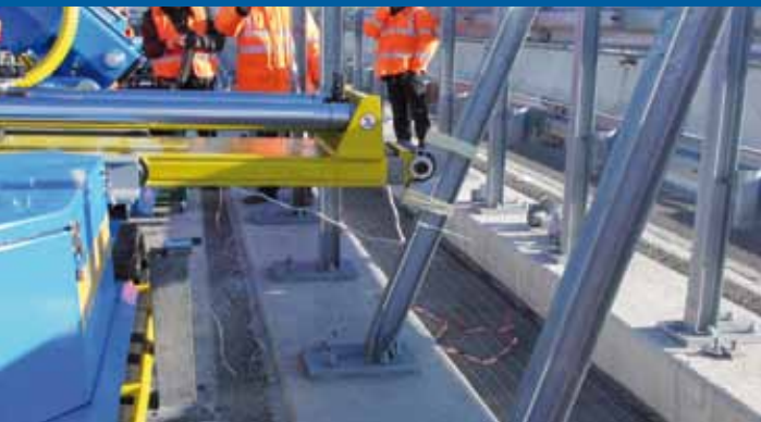
Static and Dynamic Tests on HE100A posts on rigid deck
